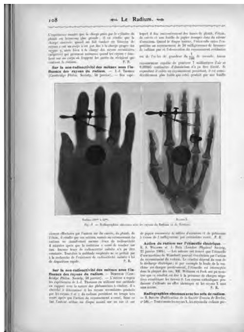
10 Comparison of radiographs made by radium and xray, Le Radium , 1905:108
